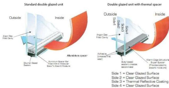
Good to know: the Resistance (R-value) of a window results of the combination for the R-value of the frame and the R-value of the glass. Thermally broken frame with double glazed glass (with thermal spacer) is a must have with new building.
